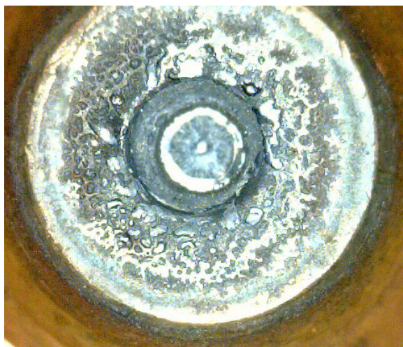
Figure 64 – Non-symmetrical, rough-edged pit and rough-surfaced electrode face
